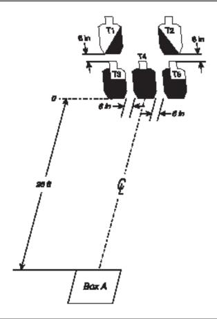
SETUP NOTES: Targets T1 & T3 and T2 & T5 are mounted above each other on one target stand. The bottoms of T3, T4, and T5 are 14 inches above ground.
